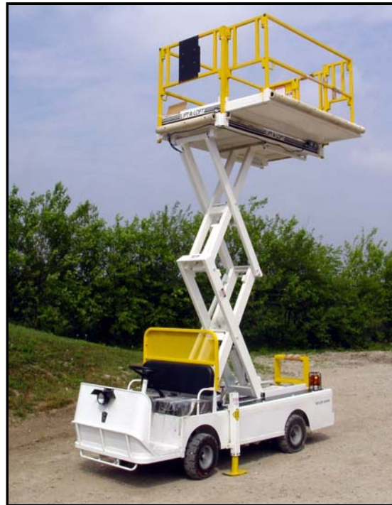
MP Scissor Lift Mounted on Burden Carrier
