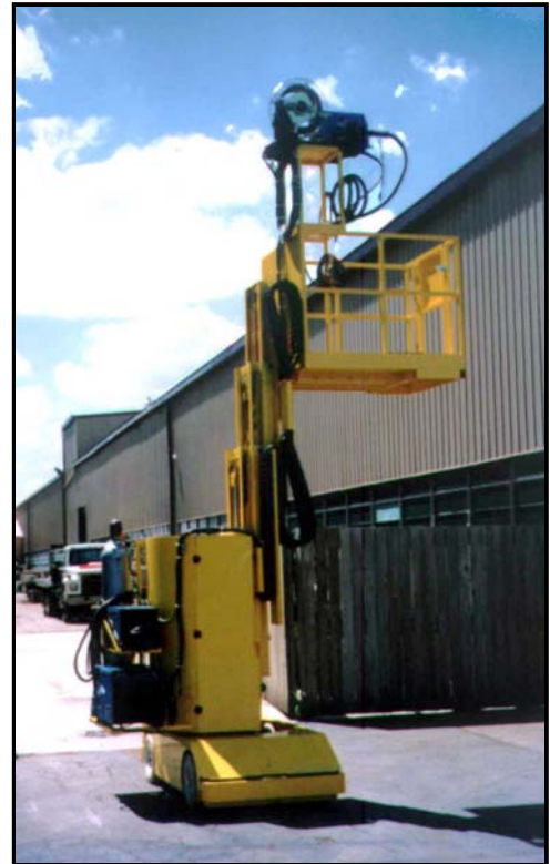
AMV with Portable Wire Feed Welder
